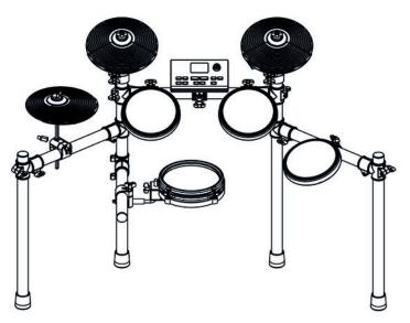
**5.** Insert the rod of the sound module holder into the clamp on the frame and tighten the wing nut.
