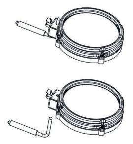
**3.** Attach the angle pieces to the Snare drum pad and the Tom drum pads and tighten the wing nuts.
