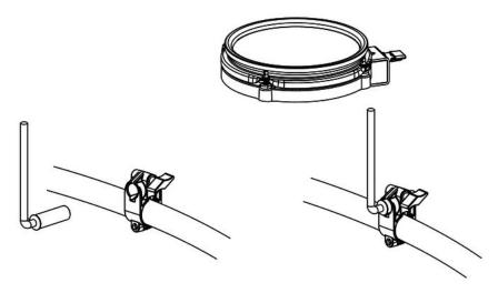
Attach the angle pieces to the brackets. Insert the snare pad and the tom pads into the angle pieces and tighten the wing nuts.
