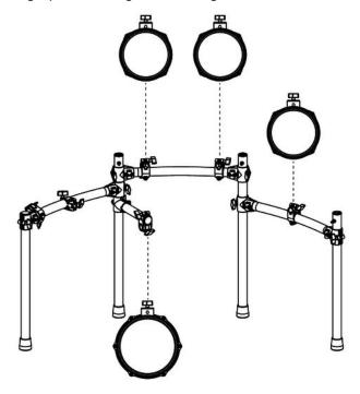
**4.** Attach the pads to the frame on the locations shown in the illustration.
