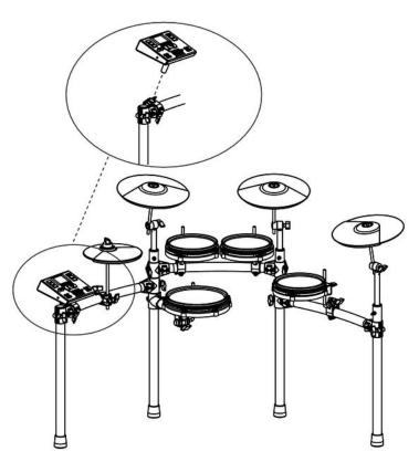
**5.** Insert the rod of the drum module holder into the clamp on the frame and tighten the wing nut.
