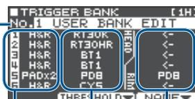
Trigger type (head)      Trigger type (rim)
