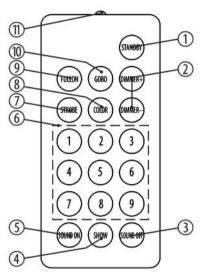
To use the remote control, point its infrared diode at the infrared sensor on the unit and press the desired buttons. The maximum operating distance is about 9 m. The device will only respond to the remote control signals if it is not controlled via DMX.
