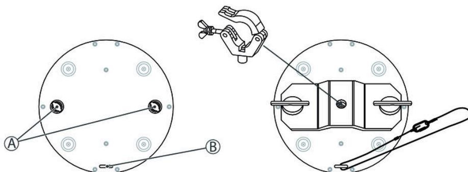
A Quick lock openings for Omega brackets
