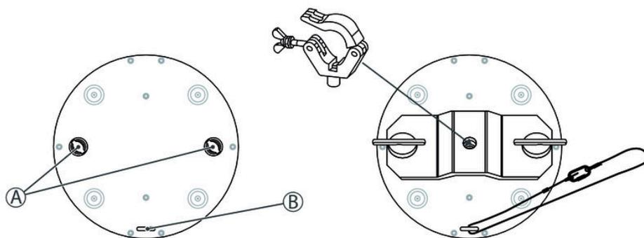
A Quick lock openings for Omega brackets
