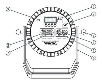
Display and keypad [MENU] Activates the main menu, changes between menu levels or closes a submenu. [DOWN] Decreases the displayed value by one. [UP] Increases the displayed value by one. [ENTER] Opens a submenu or confirms a value. 2 Pressure compensation element 3 Locking screws for the brackets. 4 [DMX IN] DMX input, designed as 3-pin XLR chassis-mounted plug (IP65)
