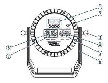
Display and keypad [MENU] Activates the main menu, changes between menu levels or closes a submenu. [DOWN] Decreases the displayed value by one. [UP] Increases the displayed value by one. [ENTER] Opens a submenu or confirms a value. 2 Pressure compensation element 3 Locking screws for the brackets. 4 [DMX IN] DMX input, designed as 3-pin XLR chassis-mounted plug (IP65)
