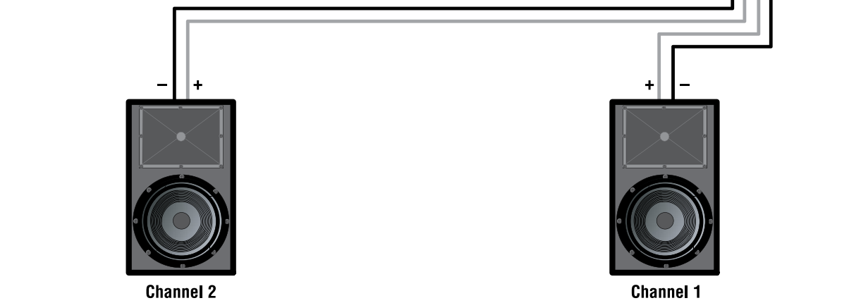
Figure 2.11 Stereo Wiring Using Both Speakon® Connectors
