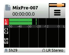
Switching between the three main meter views is easy—just touch the meters and cycle through the different views. The meters will show not only signal levels, but also the current arm status of each track for the recorder and limiting activity for L,R and each channel.
