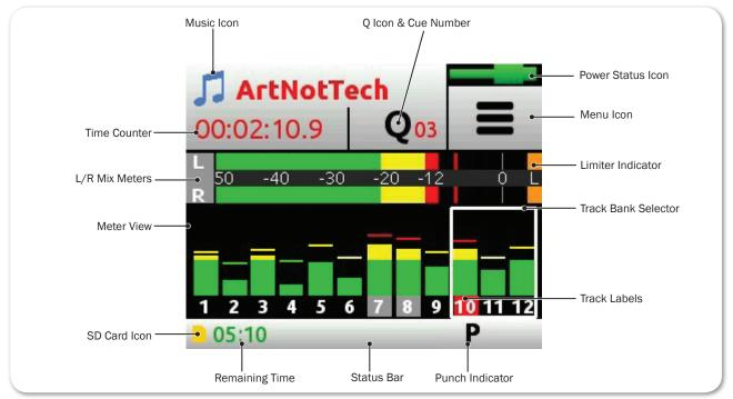
(1) The sample image shows the Home screen on a MixPre-3, as indicated by the Track Bank Selector (white box) being around only three meters. This appears differently on the MixPre-6 and MixPre-10T.
