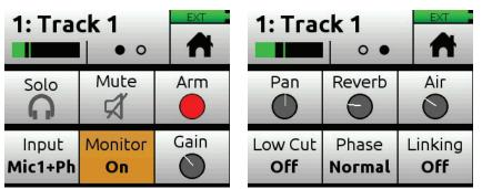
Each Channel screen provides two pages of settings—indicated by Dots icon. Tap the Dots icon to switch pages.
