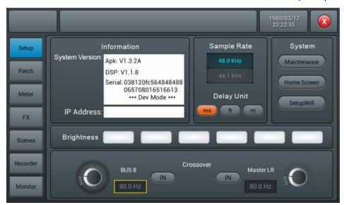
Press [SetupWifi]. When the WiFi module is connected to the device, the following screen appears.
