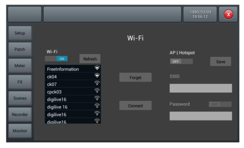
If necessary, activate the WiFi function [WiFi - ON] and tap on the corresponding list entry to select a network. Press [Connect] to establish the connection. With [Refresh] a new network search is carried out, with [Forget] you remove the marked net from the list.
