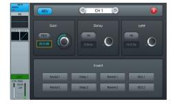
Open the transmission settings and send the selected channel to one of the 4 stereo buses [Bus5]...[Bus8]. Turn off the transmission to [LR].
