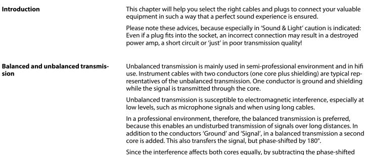
Since the interference affects both cores equally, by subtracting the phase-shifted signals, the interfering signal is completely neutralized. The result is a pure signal without any noise interference.
