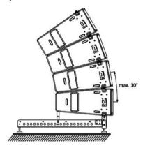
Usually, several units are so installed to a line array, that they are arranged arcuately. The figure alongside shows an example of how four elements can be combined into a system that stands on the ground (ground stack).
