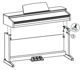
Put the digital piano housing on the stand and affix it using four hand screws.
