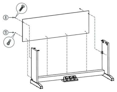
Attach the rear panel to the pedal box with four screws  $4 \times 15$  and with two screws M6  $\times$  18 to the mounting brackets of the side panels.
