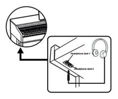
To the left beneath the keyboard you find the headphones outlets 1 and 2 (designed as 1/4" phone socket).
