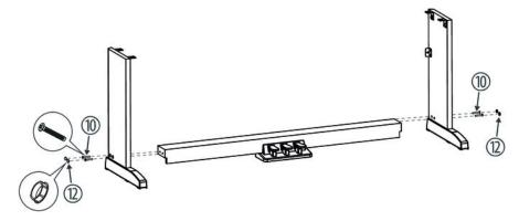
Put the pedal box between the left and right side panel and use two screws  $6 \times 50$  on each side to affix both side panels to the pedal box. Attach the four plastic caps.
