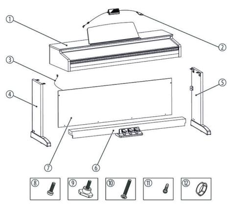
You need a Phillips screwdriver (not supplied) for the assembly of the digital piano. Open the package and make sure before assembling that the entire scope of delivery is present, as posted here.
