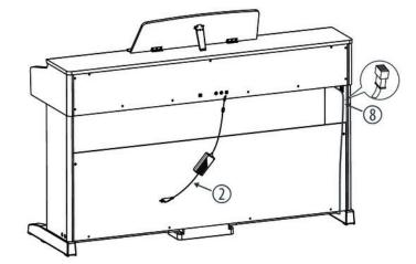
Connect the DIN plug of the pedal cable to the provided socket on the bottom side of the digital piano housing. Fix the cable to the base and move the digital piano to the desired position.
