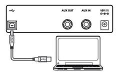
You can connect the digital piano to exchange data with a PC via the USB port. This also allows the transfer of MIDI data.
