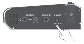
Turn on the power in the order of source devices → output devices.
