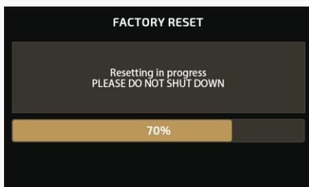
After continuing with the factory reset, this screen will appear showing that reset is in progress. Do not disconnect the power supply while the reset is in progress. Disconnecting the power supply may cause Ampero to malfunction.
