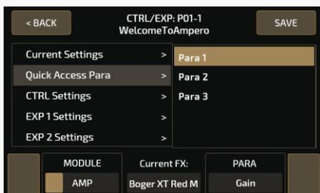
Use quick access knob 1 to select the target module. If you don't want the quick access knob on, select OFF to turn its function off. When a quick access knob is off, the parameter panel will display the status as shown:
