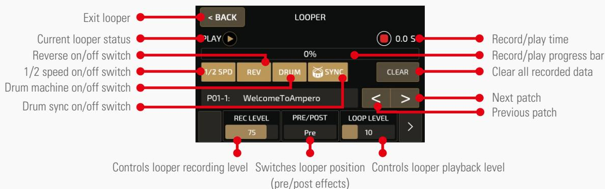
The progress bar at the top will be shown in red during recording and overdubbing. It will be shown in green in play mode.
