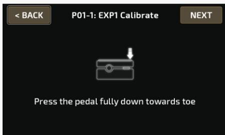
Then press the pedal all the way down and press NEXT.
