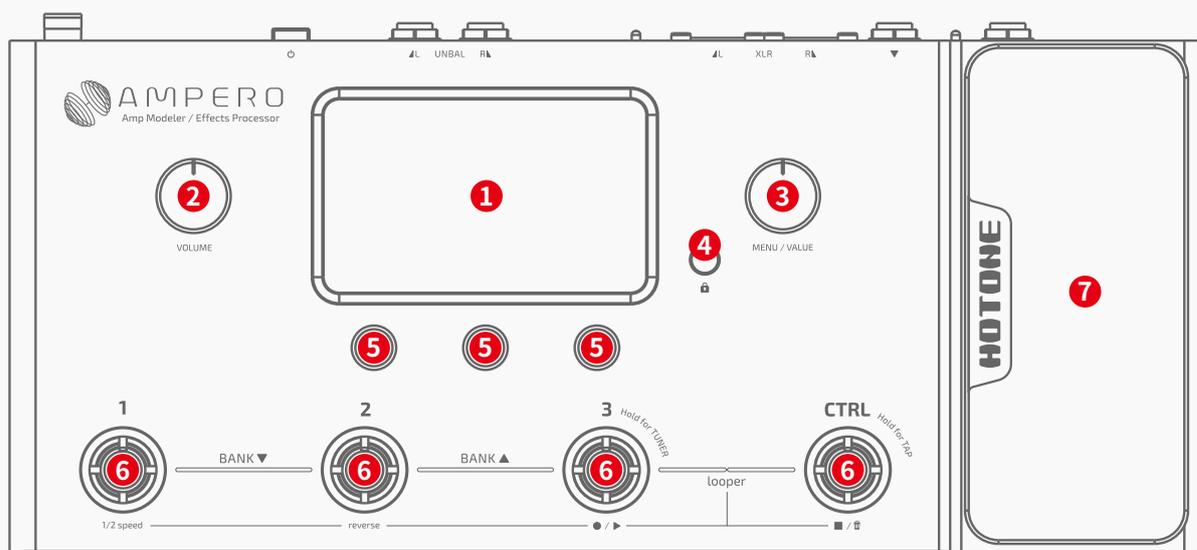
**1. Display Screen:** Displays Ampero’s current status. Use the touchscreen to select effects, edit patches, and make tone adjustments.
