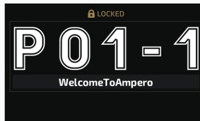
After you hold the lock icon on the screen or press the lock button on the device, Ampero will be locked. The screen will display like this.
