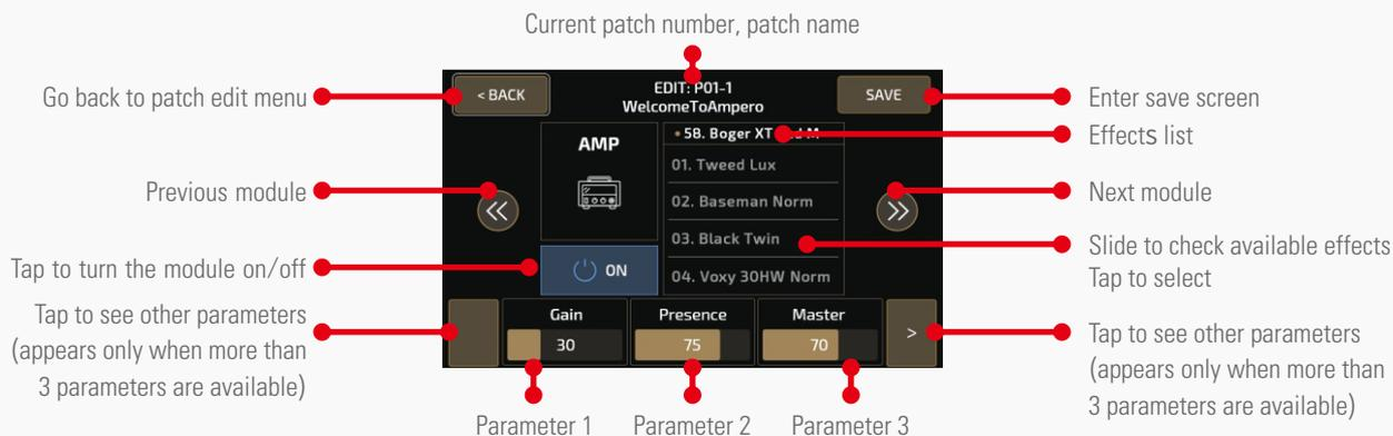
Use the module control panel to edit or turn the current module on/off.
