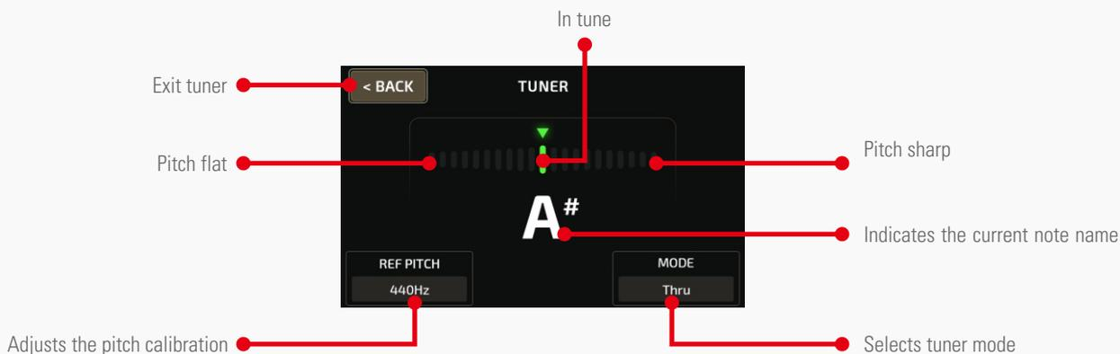
On the upper part is a scale that indicates your pitch. Left of center is flat, and right of center is sharp. As you tune your instrument towards the middle, the color of the scale will change from red (out of tune) to yellow (near pitch) to green (in tune).
