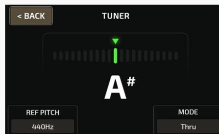
When finished, tap the footswitch again to exit the tuner.
