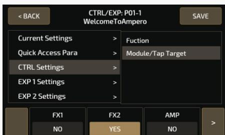
The 9 Ampero effects modules are listed in the panel, with yes and no below each module to show if the CTRL footswitch is activated or not. In the example image above, FX1, FX2 and AMP modules are controlled by the CTRL footswitch.
