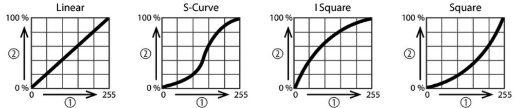
The figure schematically shows the adjustable dimmer curves. Depending on the selected DMX value (1) the device lights with a brightness (2) between 0 % and 100 %.
