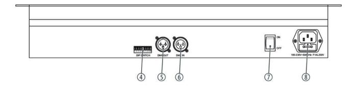
4 DIP switch for setting the DMX address
