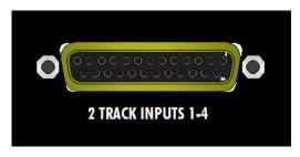
**2 TRACK INPUTS 1-4**: External stereo monitor and cue sources
