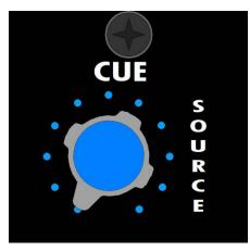
**CUE SOURCE** selections are additive, so more than one source can be selected. Each source is added in stereo at unity gain. **CUE SOURCE** selections are fed to the **CUE MASTER** via the **CUE SOURCE** level control.
