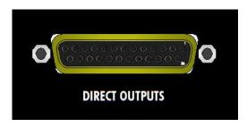
**DIRECT OUTPUTS**: Direct outputs from input channels 1-8
