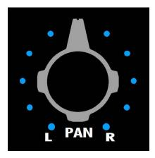
**PAN (Pan-pot)**: Continuously variable stereo (left-right) pan-pot
