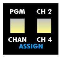
Engaging the **PGM-CHAN** switch on Compressor 2 will move Compressor 2 from the right side of the program bus to input channel 2 by default. Engaging **CH 4** will assign Compressor 2 to input channel 4. These switches illuminate when engaged.
