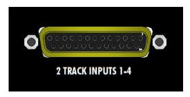
**<u>2 TRACK INPUTS 1-4</u>**: External stereo monitor and cue sources
