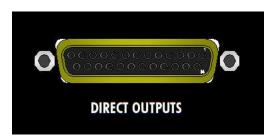
**<u>DIRECT OUTPUTS</u>**: Line-level direct outputs from input channels 1-8
