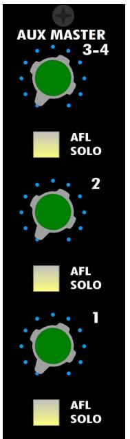
AUX MASTER 3-4: Output level control for auxiliary buses 3 & 4
