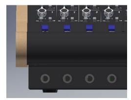
**INST IN:** Instrument-level preamp input
