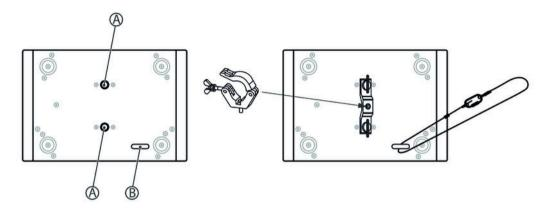
The threads on the bottom side of the housing (A) allow the secure attachment of the included mounting bracket. There, you can fasten adapters such as half couplers, trigger clamps, chooks etc. Safety cables are being threaded through the eyelet (B) on the bottom side of the housing.
