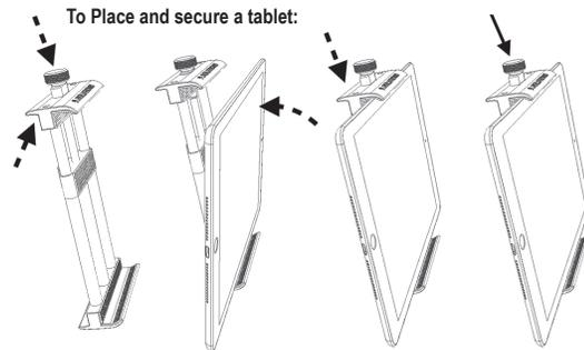
Hold against knob with thumb while lifting the jaw with other fingers.
