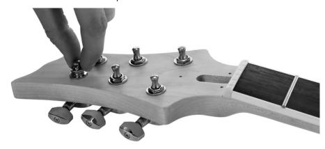
Tighten the nuts on the front with an appropriate spanner, then tighten the screws on the back firmly to fasten the tuners.
