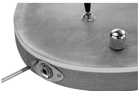
Then screw the holder of the output socket to the body with the screws provided.
