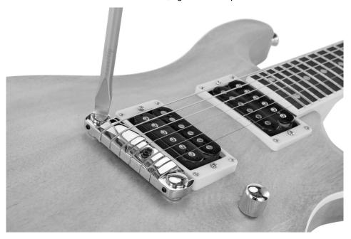
Use the two Allen screws on the tailpiece to adjust the strings action according to your playing habits, using the hexagon wrench provided. Again, the lower the string action, the easier the strings are to grip, but cause slight background noise when playing the guitar.
