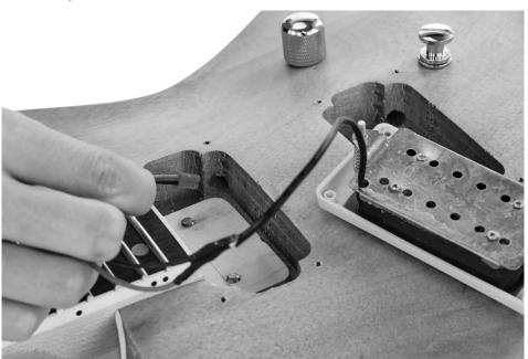
Turn the guitar over and attach the pick-ups to the front recesses with the supplied screws.
