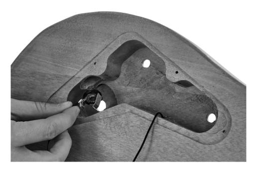
Insert the switch into the recess provided at the back.
