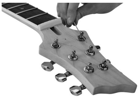
Then tune all the strings in sequence to the correct pitch. You can use a tuner or a pitch pipe as a reference. Note that the string tension will drop a little and the guitar needs to be retuned several times until the strings stay in tune.
