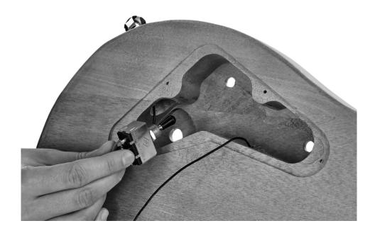
Insert the pots into the back slots as shown in the following illustrations.
