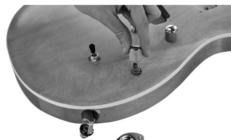
Press the pot knobs on the pins of the two pots.
