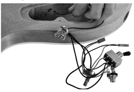
Pull the cable far enough out of the hole that there will be sufficient contact with the metallic surface when the tailpiece is installed. Earthing the strings reduces noise (humming).
