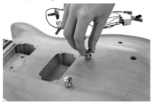
Lead the output socket from the back of the body through the hole provided on the body edge.
