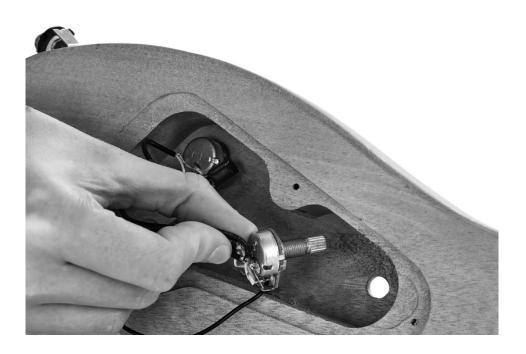
Turn the guitar over and fix the pots and switch with the supplied washers and nuts on the front of the body.
