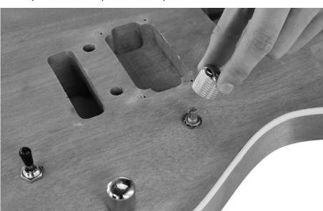
Press the pot knobs on the pins of the two pots.
