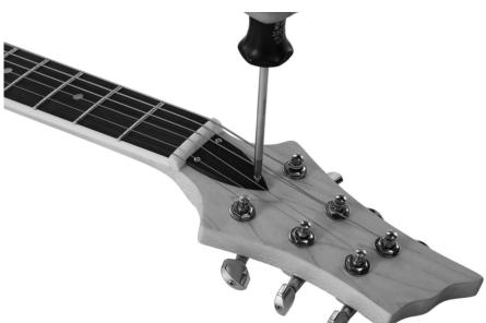
Screw the truss rod cover onto the headstock.
