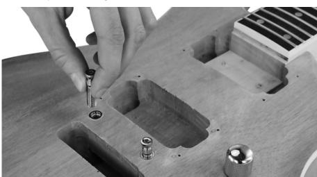
Screw the tailpiece mounting bolts into the bracket.
