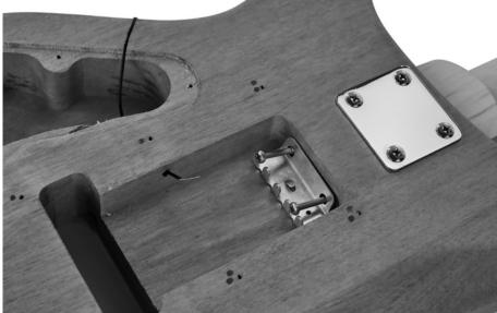
Attach the earthing cable to the pre-assembled spring plate. Make sure there is sufficient contact between the stripped end of the grounding cable and the spring plate.
