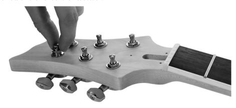
Tighten the nuts on the front with a suitable wrench, and then tighten the screws to secure the machine heads on the rear side.
