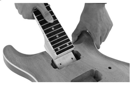
Turn the guitar over, position the mounting plate over the four screw holes on the back of the body and screw the four supplied long wood screws through the holes in the mounting plate into the body and neck until the connection is firm.
