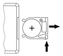
Press the lock of the battery holder to the centre of the housing and pull out the battery holder like a drawer. Insert the battery. The battery is correct if the positive pole points to the housing base of the remote control. Slide the battery holder back into the remote until it clicks into place.
