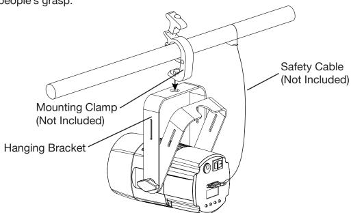
**NOTE:** This unit comes with 2 velcro safety straps. It is highly suggested that both straps are used to properly secure the unit.
