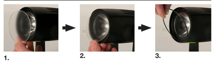
The Saber Spot GO comes with 2 frost filters. Before installation, peel off the adhesive backing on both sides of the lens. Install the frost filter in front of the main lens (1 & 2). Insert the inlcuded retainer ring by "squeezing" the ring and gently sliding it in place in front of the newly installed lens (3).
