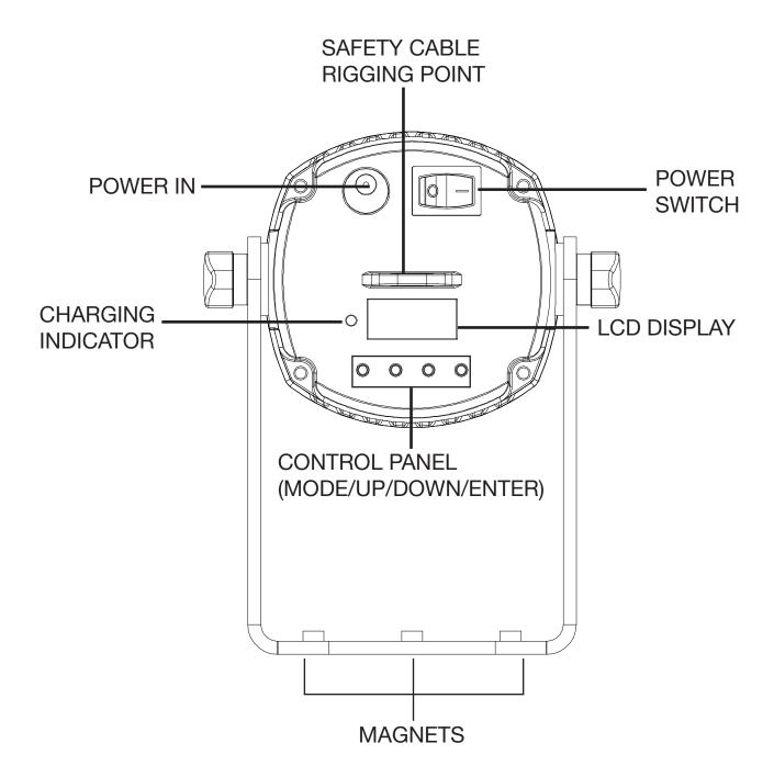
All fixtures should be given a DMX starting address when using a DMX controller, so the correct fixture responds to the correct control signal. This digital starting address is the channel number from which the fixture starts to "listen" to the digital control signal sent out from the DMX controller. The assignment of this starting DMX address is achieved by setting the correct DMX address on the digital control display on the fixture.
