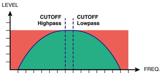
Figure 4: Bandpass filter: the green area is being passed through the filter whereas the red area is rejected.
