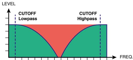
Figure 6: Notch filter: The green area is being passed through the filter whereas the red area is rejected.
