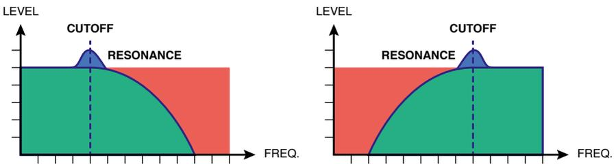
Figure 2: Left: lowpass filter with resonance, Right: highpass filter with resonance;
