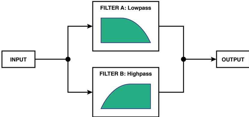
Figure 5: Parallel combination of low- and highpass filter
