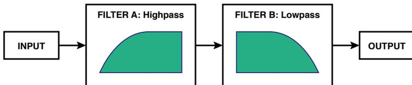
Figure 3: Serial combination of high- and lowpass filter
