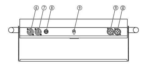
6 [POWER IN] Lockable input socket (Power Twist) for powering the device 7 [POWER OUT] Lockable output socket (Power Twist) for powering further devices 8 [F2AL250V] Fuse 9 Safety eye for attaching the safety cable 10 Display [MENU] Activates the main menu for selecting the operating mode  $\blacktriangle$ Increases the displayed value by one Decreases the displayed value by one
