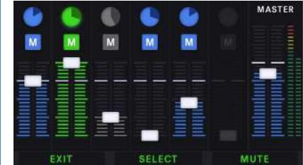
**On-screen label text** describes the SINGLE TAP commands of the bottom three buttons
