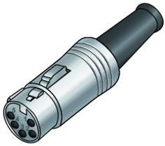
A five-pin XLR socket serves as DMX output, a five-pin XLR plug serves as DMX input. The drawing below and the table show the pin assignment of a matching coupling.
