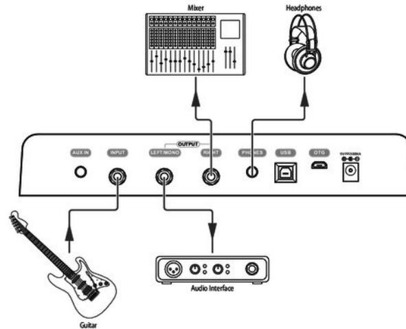
1. ➤ Connect the guitar to the input jack [INPUT] of the unit.
