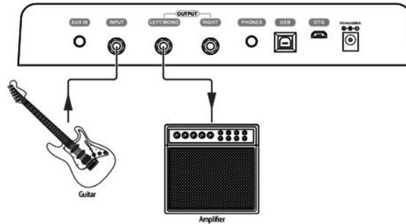
1. ➤ Connect the guitar to the input jack [INPUT] of the unit.
