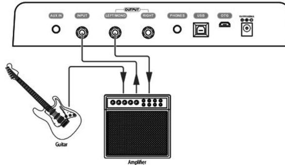
1. ➤ Connect the guitar to the input of an amplifier.
