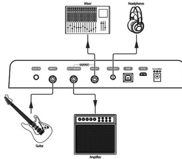
1. ➤ Connect the guitar to the input jack [INPUT] of the unit.
