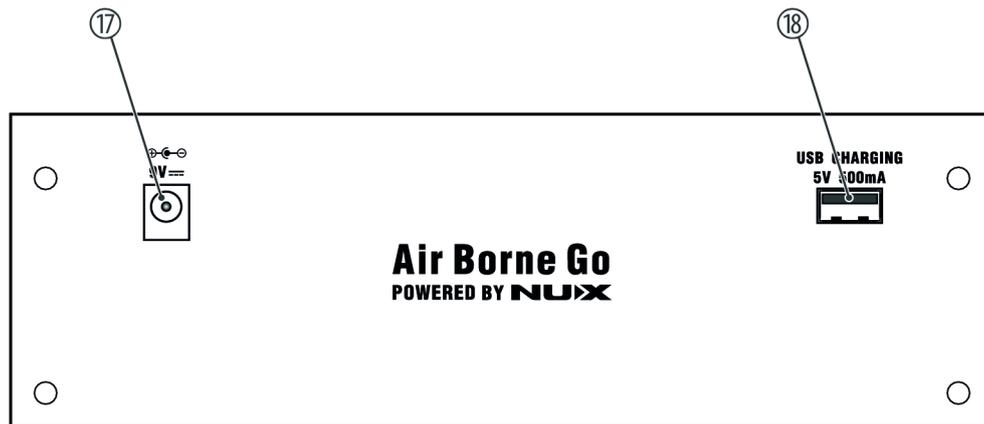
17 Socket for connecting the supplied plug-in power supply
