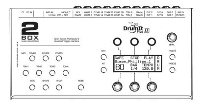
The main page comprises six logical areas. The three DATA buttons above the display are assigned to the values or functions that appear in the top row. Press the button above the desired entry to set values or select functions. However, please use the three rotary knobs below the display to change the according parameter values in the bottom row.
