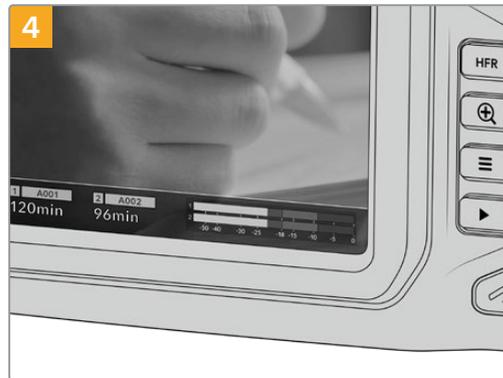
The storage information at the bottom of the LCD touchscreen will show the name and record time remaining of the detected SD card.
