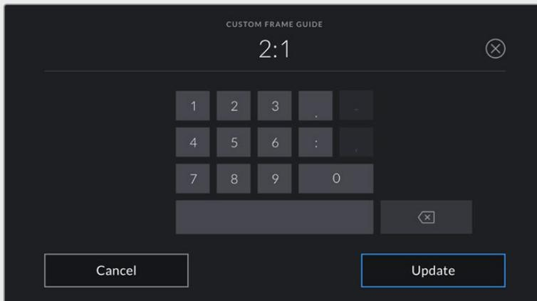
Use the numeric keypad on the 'custom frame guide' screen to enter a new frame guide ratio
