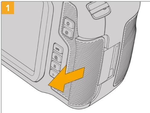
To access the media slots, slide the door on the right side toward the back of the camera.
