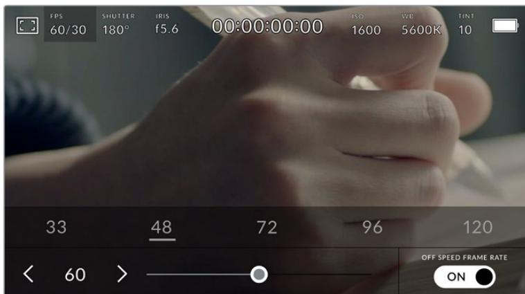
With 'off speed frame rate' enabled, tap a preset or the arrows on either side of the sensor frame rate or move the slider to make adjustments
