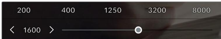
While in the 'ISO' menu, your camera's ISO settings appear along the bottom of the LCD touchscreen. The slider below the presets lets you adjust ISO in 1/3 stop increments.
