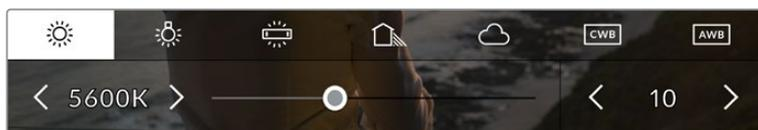
Tapping the white balance and tint indicator gives you access to five presets, as well as a white balance indicator and slider on the left, and a tint indicator on the right. Adjust these to set a custom white balance for your lighting conditions
