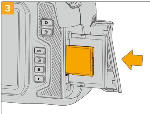
With the label on the SD card facing the touchscreen, insert the SD card into the SD card slot until you feel it lock into place. The card should insert easily without the need for excessive force.
