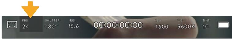
Tap the frames per second indicator to access frame rate settings
