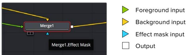
Multiple outputs on nodes means a single node can connect to many different nodes in your composition, so you don't have to duplicate clips as you would in layer based software. Arrows on the line between connected nodes are a great visual indicator to show you which direction the image data is flowing.
