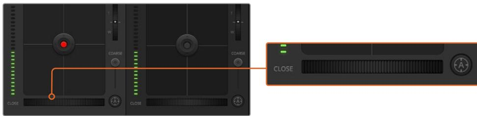
Click on the auto focus button or drag the manual focus adjustment left or right to focus a compatible lens.
