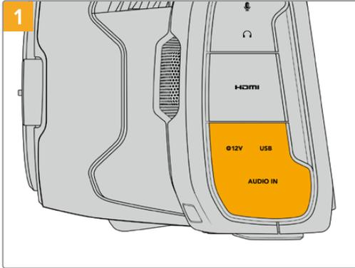
1 Open the rubber protector on the left side of the camera and connect the other end of the cable to the USB-C port.
