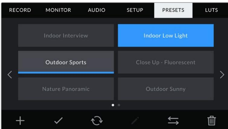
Select a preset and tap the 'load' icon to load it. Selected presets will appear solid blue, while currently loaded presets have a blue line along the bottom of their icon
