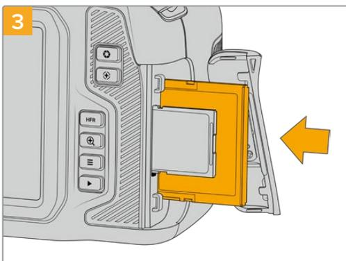
Insert the CFast card into the CFast card slot until you feel it lock into place. The card should insert easily without the need for excessive force. To remove a CFast card, gently push the CFast card in and then release to eject it.
