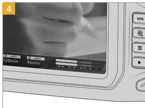
The storage information at the bottom of the LCD touchscreen will show the name and record time remaining of the detected CFast card.
