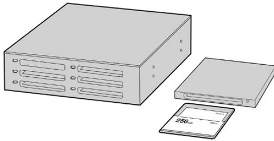
Edit directly from your CFast or SD card by removing it from your camera and mounting it on your computer using a CFast 2.0 reader/writer or CFast drive
