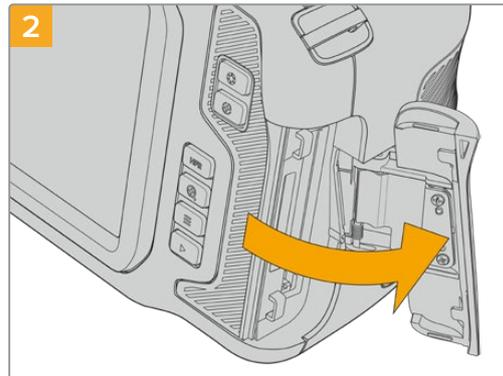
The spring loaded door opens so you can access the CFast and SD memory card slots.
