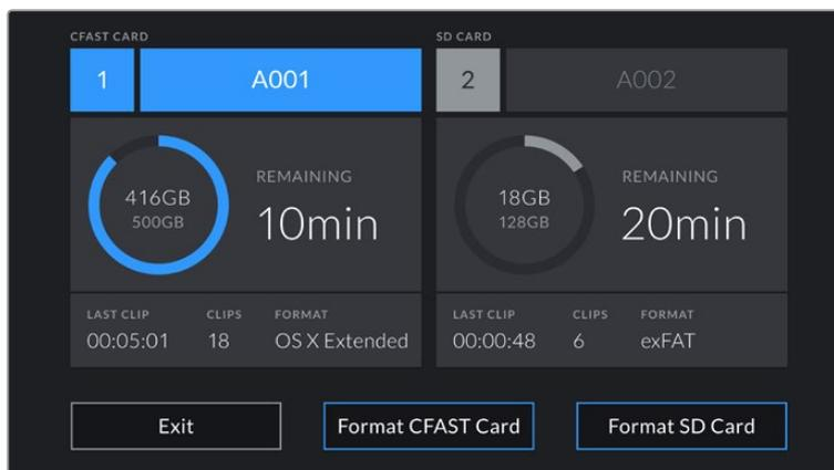
'Format SD card' is replaced with 'Format external drive' in your storage and formatting screen when you have a USB-C flash disk connected to your camera
