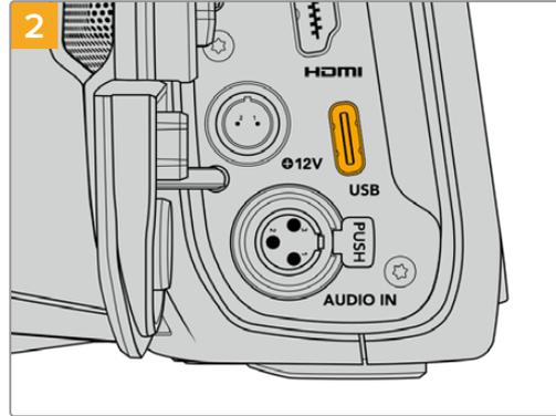
2 Connect one end of a USB type-C cable to your USB-C flash disk.
