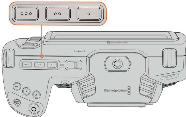
The function buttons are represented by dots and are located on the top of your camera
