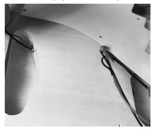
Connect the pickup connector to the connectors for the control plate. Insert the output jack into the hole provided on the edge of the guitar body.
