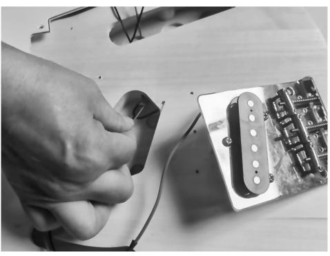
Run the cable for earthing the strings (stripped, without connectors) through the channel in the recess for the control plate and into the recess for the bridge pickup.
