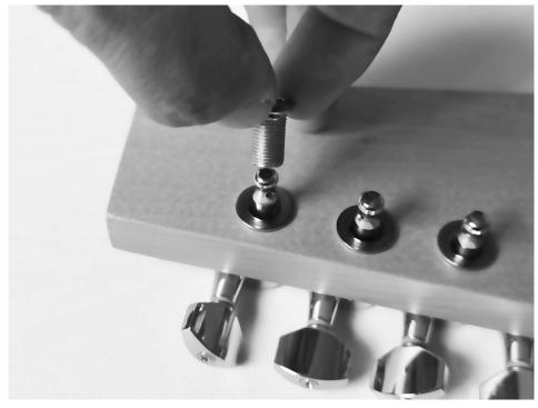
Tighten the nuts on the front with a suitable wrench, and then tighten the screws to secure the machine heads on the rear side.
