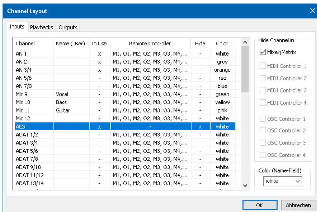
The dialog can be called directly from TotalMix by a right mouse click on any channel. The corresponding channel will then be preselected in the dialog.
