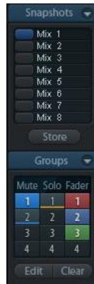
TotalMix uses flashing signals to guide you through the group setup. After a click on Edit and click on the desired storage place all desired functions for this group have to be activated or selected. The storage process is finished by another click on Edit.
