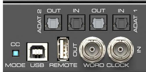
**Word Clock I/O.** BNC. The Settings dialog includes an option to activate internal termination (75 Ohms).
