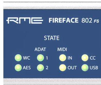
**MIDI LEDs.** Indicate separately for input and output if MIDI is received or transmitted.
