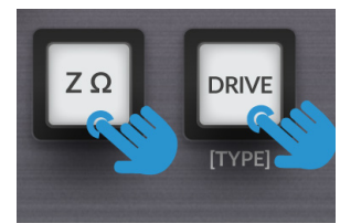
Channel 4 Buttons ZΩ decreases timeout, DRIVE increases timeout
