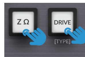
Channel 1 Buttons ZΩ decreases brightness, DRIVE increases brightness
