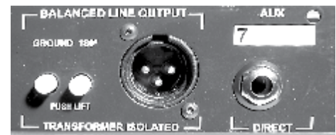
Channel-7 - Rear panel 1/4" output jack, Balanced (recording) XLR output & switches.
