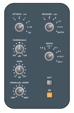
Adjust threshold for 4-5 dB G.R Adjust make-up gain accordingly
