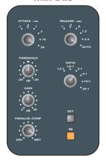
Adjust threshold for 2-3 dB G.R Adjust make-up gain accordingly
