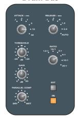
Adjust threshold for 6-8 dB G.R Adjust make-up gain accordingly
