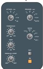
Adjust threshold for 8-10 dB G.R Adjust make-up gain accordingly
