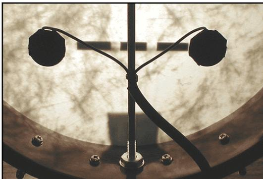
We recommend you only apply double-sided tape to the two outer edges of the pickups. We call this the “catamaran” mounting technique because the center portion of the pickup is free floating. This enhances response while reducing the adhesive surface by about 40%.
