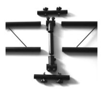
**2.** Attach the two T-pieces (B) to the ends of tube (C).
