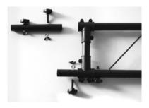
Connect the combination of (B) and (C) to the open side of one truss section (A). Then slide the tubes (D) through the T-pieces (B) into the truss section (A) and screw-connect the tubes (D).
