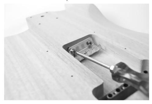
Attach the loops of the three springs to the spring claw and guide the other ends into the small holes in the sustain block. Continue to tighten the spring claw towards the neck until some tension is applied to the bridge.
