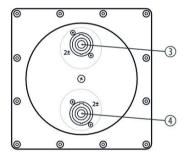
3, 4 NL4 connections, wired in parallel (2+/2- to the woofer; 1+/1- interconnected)
