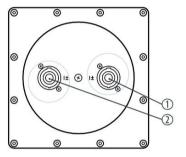
1, 2 NL4 connections, wired in parallel (1+/1– to woofer; 2+/ 2– interconnected)
