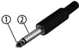
Drawing and table indicate the pin assignment of a 1/4" TS phone plug to be used.
