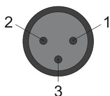
A 3-pin XLR socket is used as DMX output. The following diagram and table show the pin assignment of the XLR socket.
