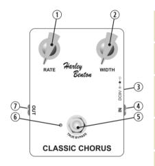
1 **RATE**Turn this knob clockwise to increase the speed of the effect.
