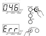
Press [SAVE] to open the SAVE menu. You can now assign the current settings to a user kit number using [SELECT -/+]. During this process the display value flashes on the three-digit LED display.
