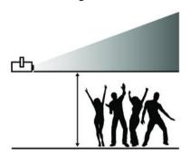
When installing the unit, observe the specified minimum height to prevent the risk of injury to persons, and observe the limits for maximum exposure of eyes or skin to a laser.
