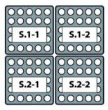
In the master-slave configuration, you can interconnect four devices of the same type to one large matrix with  $10 \times 10$  LEDs. The effects then use this device combination in common.
