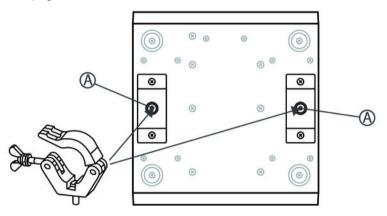
A Threads for adapters such as half couplers, trigger clamps, c-hooks etc.
