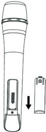
1. ➤ Make sure that the transmitter is turned off, the main switch is in 'OFF' position.
