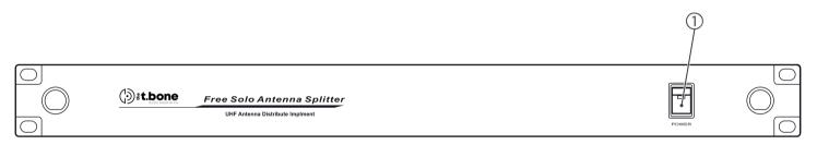
1 [POWER] | Main switch. Turns the device on and off.
